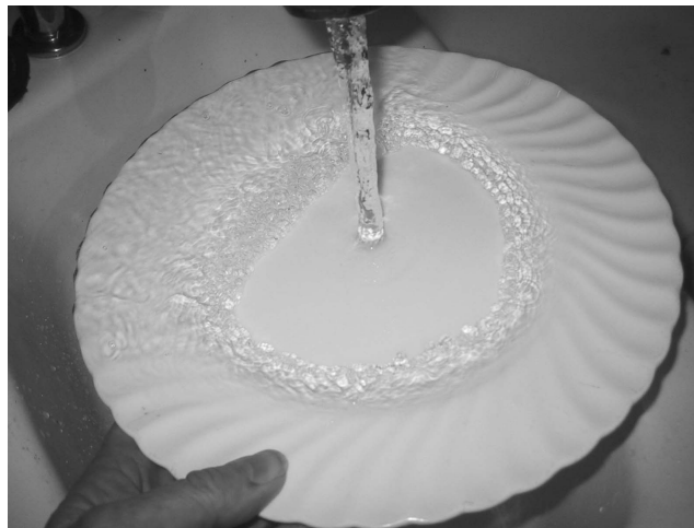
Fig. 17.14: Hydraulic jump on a dinner plate under a kitchen tap.
