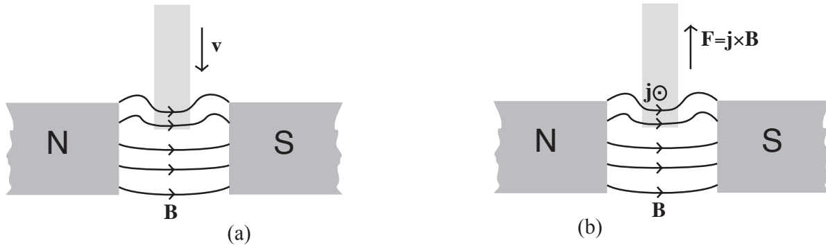
Fig. 18.1: The two key physical effects occurring in MHD. (a) A moving conductor modifies the magnetic field by appearing to drag the field lines with it. When the conductivity is infinite, the field lines appear to be frozen into the moving conductor. (b) When electric current, flowing in the conductor, crosses magnetic field lines there will be a Lorentz force, which will accelerate the fluid.
