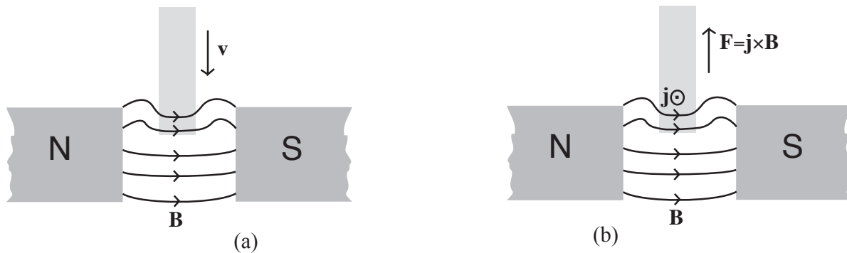
Fig. 18.1: The two key physical effects that occur in MHD. (a) A moving conductor modifies the magnetic field by appearing to drag the field lines with it. When the conductivity is infinite, the field lines appear to be frozen into the moving conductor. (b) When electric current, flowing in the conductor, crosses magnetic field lines there will be a Lorentz force, which will accelerate the fluid.
