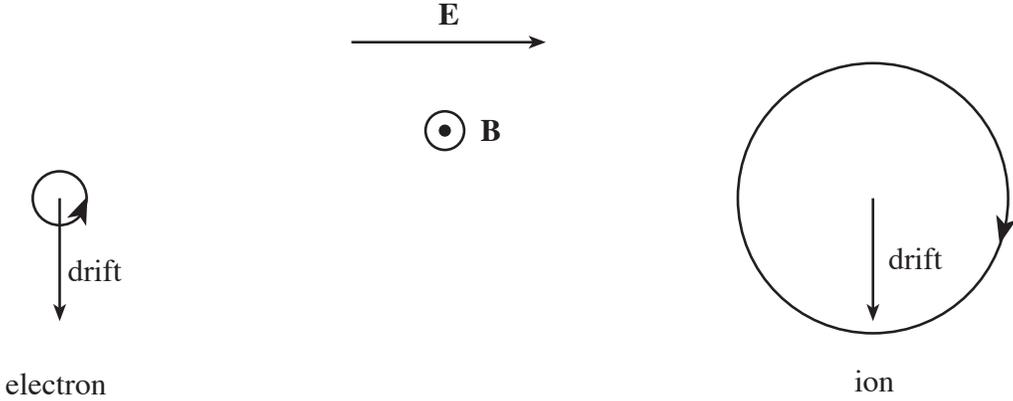
**Fig. 20.4:** Gyration of electrons and ions in a low frequency Alfvén wave. Although the electrons and ions gyrate with opposite senses about the magnetic field, their  $\mathbf{E} \times \mathbf{B}$  drifts are similar. It is only in the next highest order of approximation that a net ion current is produced parallel to the applied electric field.
