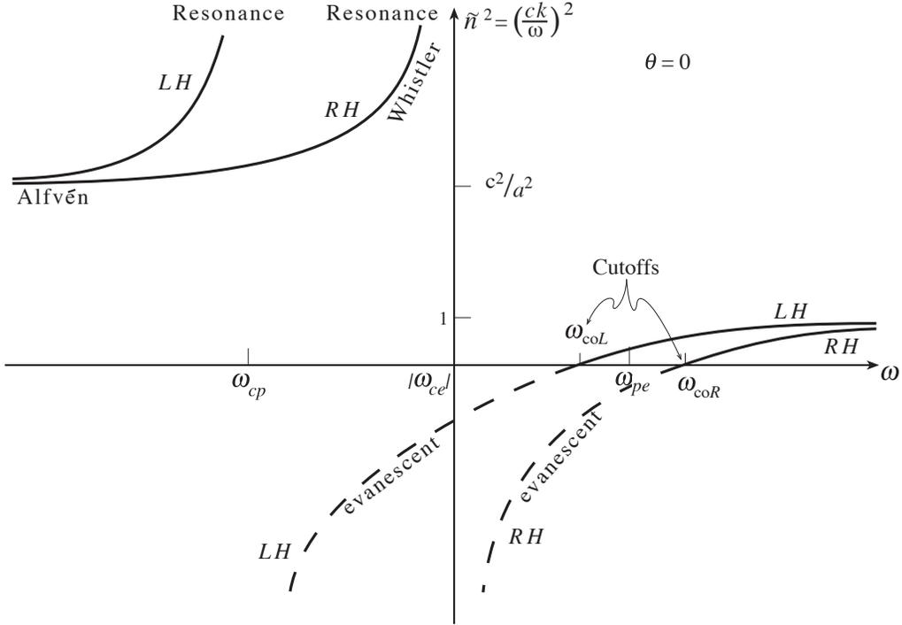
**Fig. 20.3:** Square of wave refractive index for circularly polarized waves propagating along the static magnetic field in a proton-electron plasma with  $\omega_{pe} > \omega_{ce}$ . (Remember, that we will regard both the electron and the proton cyclotron frequencies as positive numbers.) The angular frequency is plotted logarithmically in units of the modulus of the electron gyro frequency.
