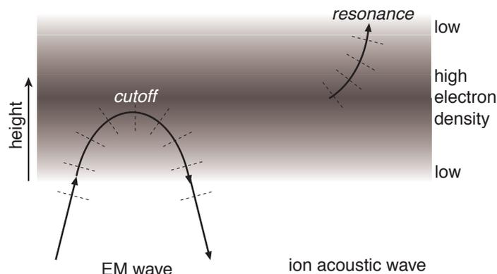
**Fig. 20.2:** Cutoff and resonance illustrated by wave propagation in the Earth’s ionosphere. The thick, arrowed curves are rays and the thin, dashed curves are phase fronts. The electron density is proportional to the darkness of the shading.
