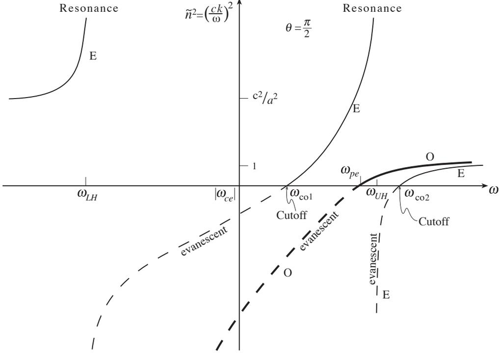
**Fig. 20.5:** Variation of refractive index  $n$  for wave propagation perpendicular to the magnetic field in an electron ion plasma with  $\omega_{pe} > \omega_{ce}$ . The ordinary mode is designated by O, the extraordinary mode by E.
