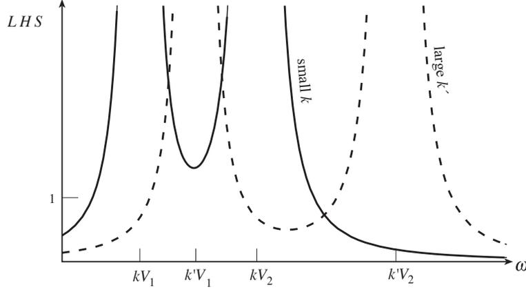
**Fig. 20.8:** Left hand side of the dispersion relation (20.77) for two cold plasma streams and two different choices of wave vector  $k$ . For small enough  $k$ , there are only two real roots for  $\omega$ .
