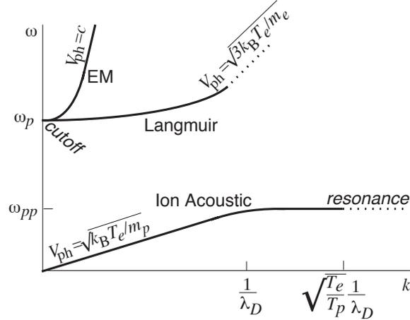
**Fig. 20.1:** Dispersion relations for electromagnetic waves, Langmuir waves, and ion-acoustic waves in an unmagnetized plasma, whose electrons are thermalized with each other at temperature  $T_e$ , and protons are thermalized at a temperature  $T_p$  that might not be equal to  $T_e$ . In the dotted regions the waves are strongly damped, according to kinetic-theory analyses in Chap. 21.
