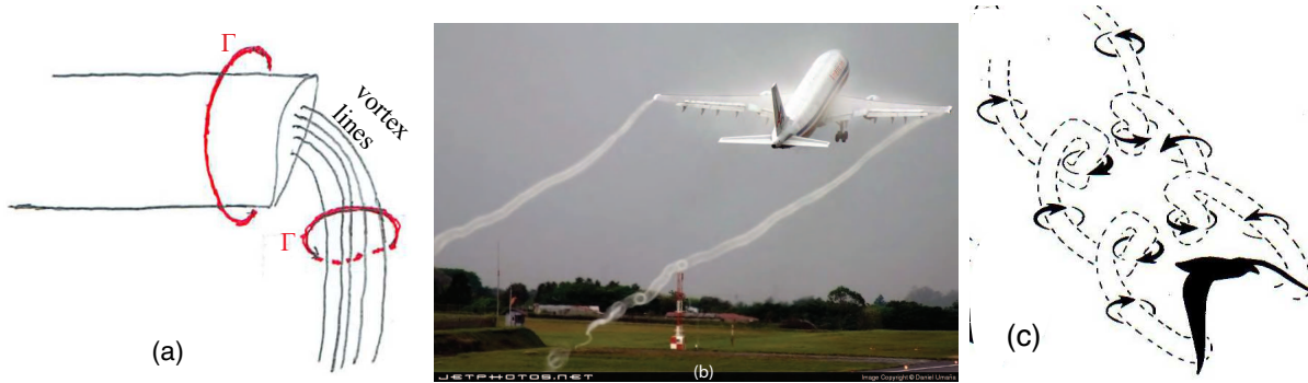
Fig. 14.2: (a) Sketch of the wing of a flying airplane, and vortex lines that emerge from the wing tip and sweep backward behind the plane. The lines are concentrated into a region with small cross section, a vortex of whirling air. The closed red curves encircle the wing and the vortex; the integral of the velocity field around these curves, \Gamma = \int \mathbf{v} \cdot d\mathbf{x} , is the circulation contained in the wing and its boundary layers, and in the vortex; see Sec. 14.2.4 below and especially Ex. 14.8. (b) Photograph of the two vortices emerging from the wingtips of an Airbus, made visible by light scattering off water droplets in the vortex cores (Ex. 14.6); photo copyright by Daniel Umaña. (c) Sketch of vortex lines (dashed) in the wingtip vortices of a forward flying bird, and flow lines (solid) of air around them; from Fig. 12.7 of Vogel (1994).
