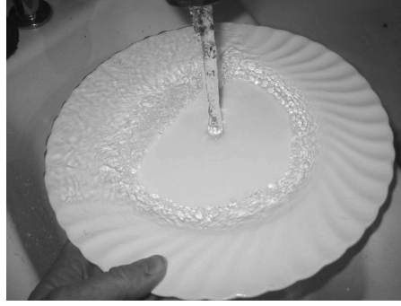
Fig. 17.12: Hydraulic jump on a dinner plate under a kitchen tap.
