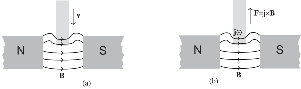
Fig. 19.1: The two key physical effects that occur in MHD. (a) A moving conductor modifies the magnetic field by appearing to drag the field lines with it. When the conductivity is infinite, the field lines appear to be frozen into the moving conductor. (b) When electric current, flowing in the conductor, crosses magnetic field lines there will be a Lorentz force, which will accelerate the fluid.
