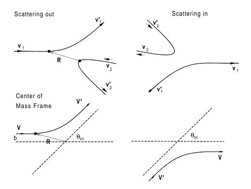
Figure 1: Binary collisions in a gas: top-lab frame; bottom-centre of mass frame
