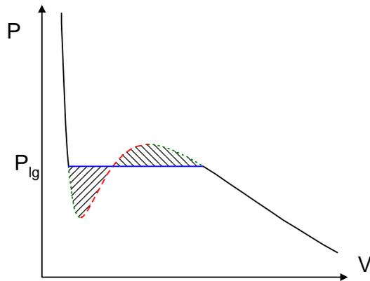
Figure 3: Maxwell construction
